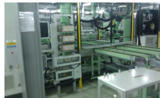
Automated busing incl. wire cutting and bowing
